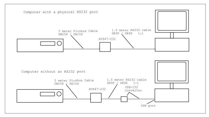
There are two ways to connect the AVS47-232/USB: Either directly to computer's RS232 port, or via a USB-232 converter to computers USB port. The USB converter creates a virtual RS232 port that your high-level program will access.
