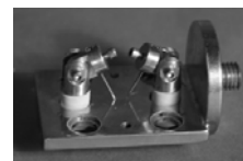
Optional Hall Probe Sample Holder. 2, 4 or 6 probes available.
