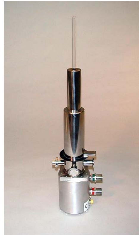
DE-202SI (4K) with DMX-15 vacuum shroud installed
