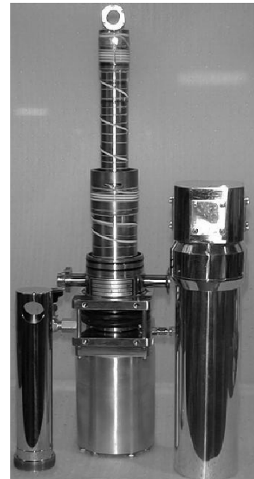
DE-204AF with interface installed. vacuum shroud and radiation shield also shown.
