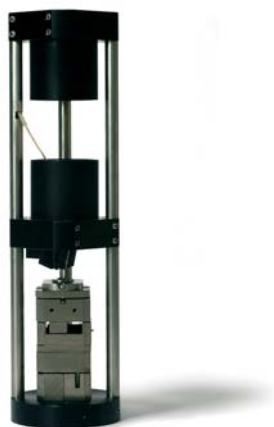
Fig. 4: The attoSNOM I microscope sensor head.
