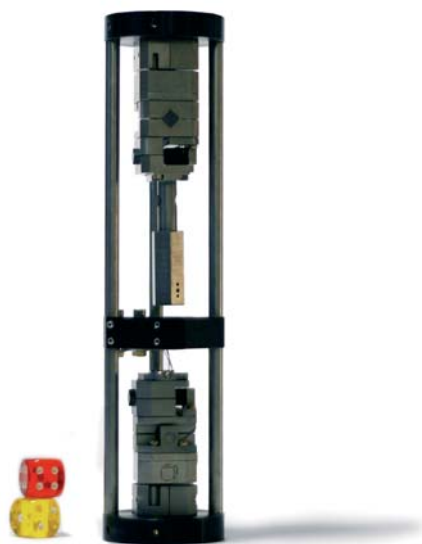
Fig. 3: The attoSNOM II microscope sensor head.
