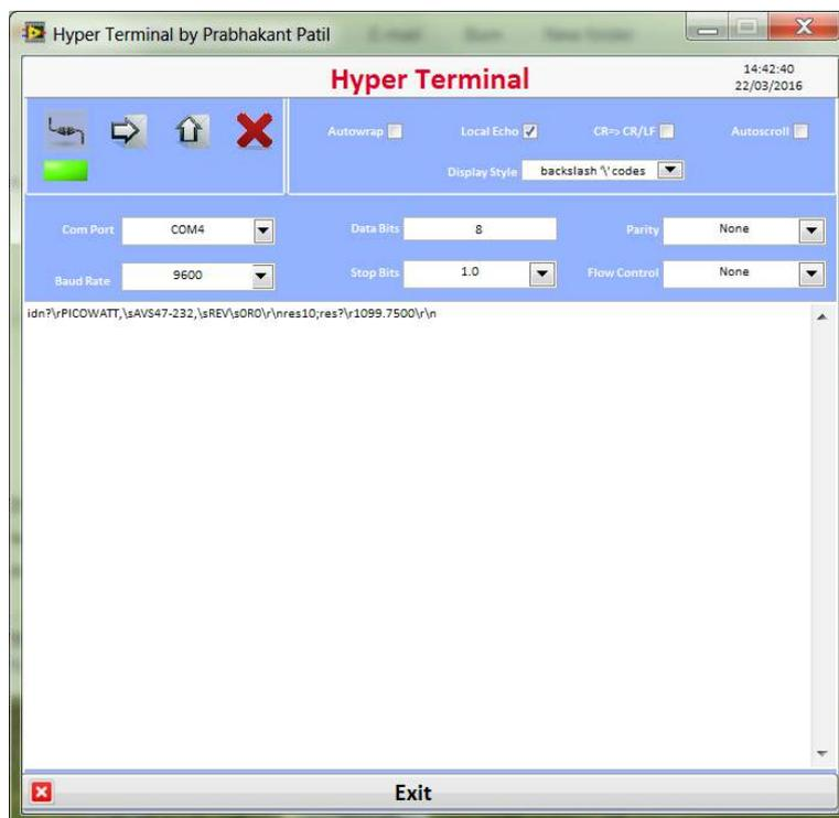
Users of LabView can also try this program (see text for link). The output includes all printing and non-printing characters in both transmitted and received strings, which can be useful for debugging. But otherwise it is far less convenient to use.
