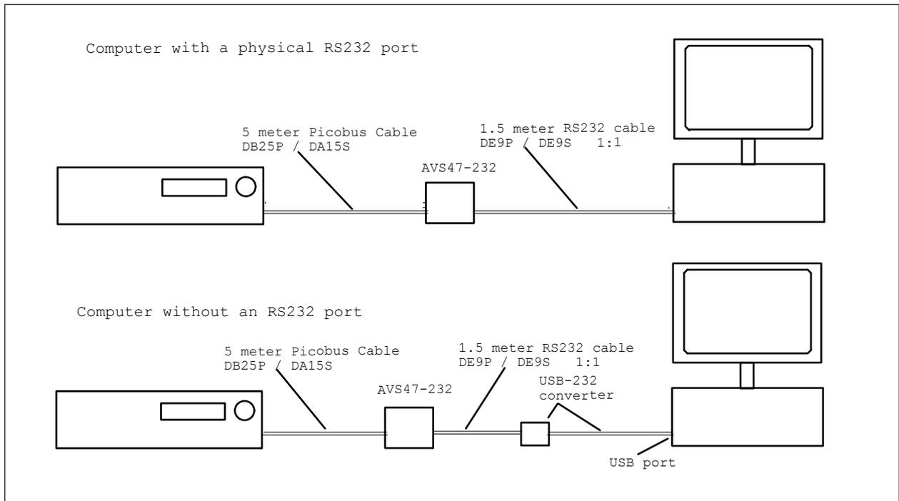
There are two ways to connect the AVS47-232/USB: Either directly to computer's RS232 port, or via a USB-232 converter to computers USB port. The converter creates a virtual RS232 port that your high-level program will access.
