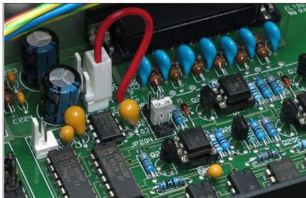
Change short circuit piece JP204 to position JP203 before making any connections in order to avoid damage to the AVS47-232/USB, which uses 0/+5V voltage levels for communications with the AVS-47B resistance bridge.
