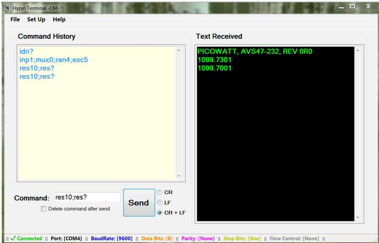
The “Hype! Terminal” (see text for link) is easy to use: Just specify the Com port number (SetUp) and it is ready. After identification, the bridge is set for measure input, channel 0, range 2k $\Omega$ , and excitation 300 $\mu$ V. Then 10 A/D conversions are taken (RES10) and the output is read by RES?. This RS232 terminal program for a Windows PC does not require LabView.
