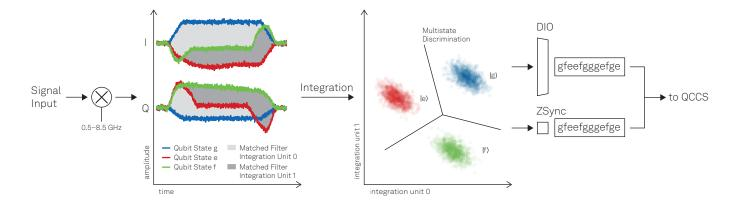
SHFQA analysis chain for a qutrit readout. After analog and digital down-conversion, the reference traces from the readout resonators are integrated using matched filters. The multi-state discrimination assigns the qubit states g, e, or f to the results and then communicates them to the QCCS in real time.
