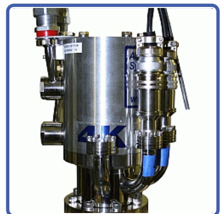
The above picture shows an instrumentation skirt with the electrical feedthroughs rotated 90 degrees upwards to allow for tight rotational clearances.
